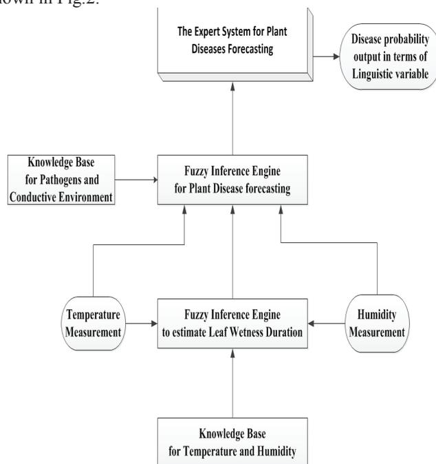
Fig. 2 Conceptual diagram of weather based plant diseases forecasting system
